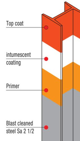
Connecting elements can be coated directly with **Sika® Unitherm®** to provide them with a 100% protection from heat.
